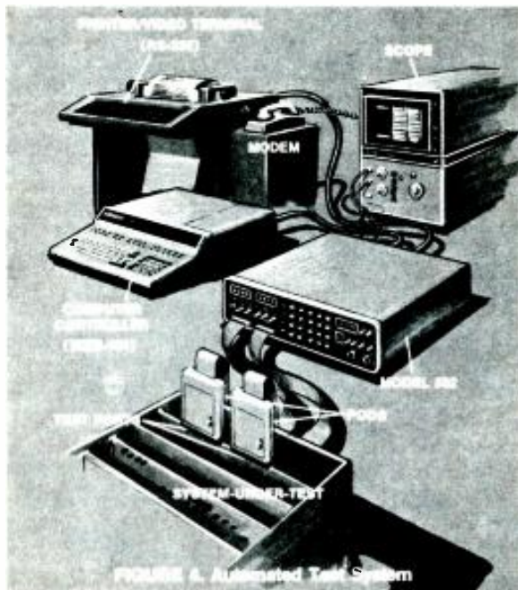
The Model 532 can interface to various output devices such as teletypes, modems, computer control devices, and scopes. Most stations will find the scope interface most useful since it provides readouts in hex or binary
